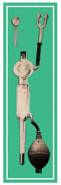
tube, or the electric sparks will not pass through the current of air supplied by the air bulb. If held by rubber handle Ozone will not be generated.
